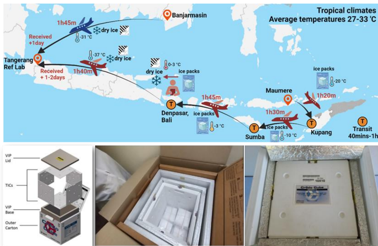
Figure 2. Specimen shipment challenges and the Credo Cube as a cold chain solution.
